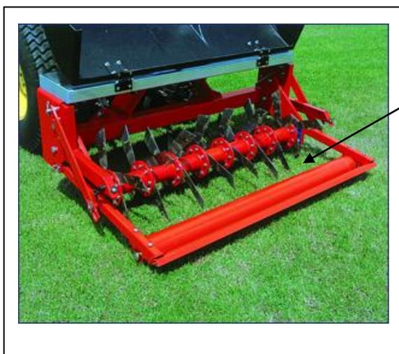
We are using a brand new large fairway slitter similar to the one shown here which works to a depth of around 10".
